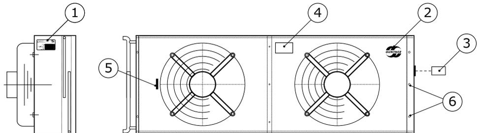
Placing of labels on the unit
