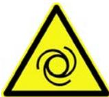
With automatic fan start during maintenance work there is a danger of pinching/trapping for the hands and fingers.
