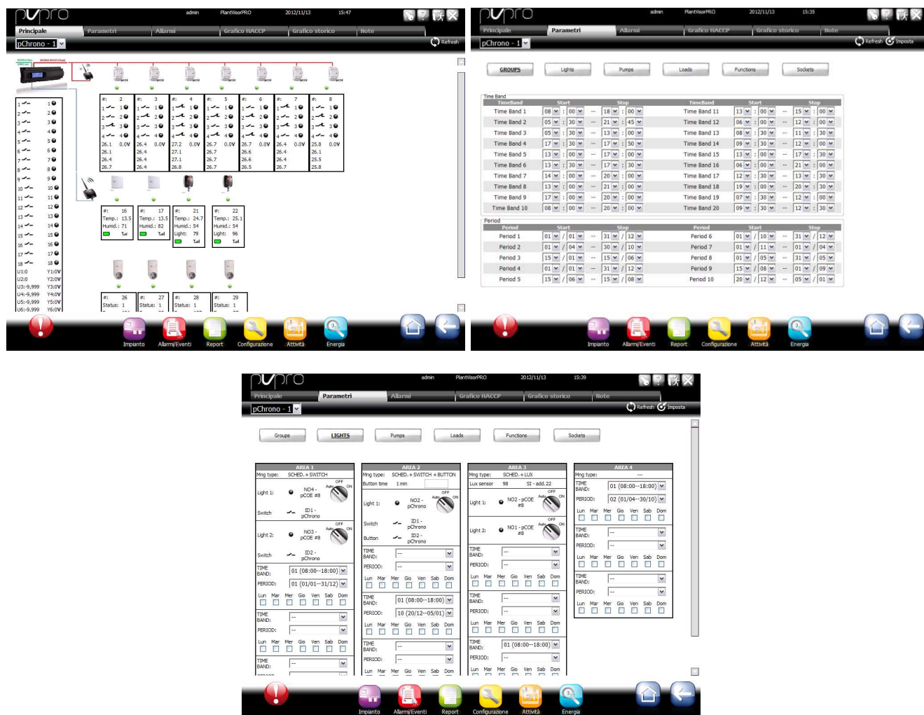
Figure 3 – Screenshots of some of the pages relating to the pChrono model. In detail: the main screen, the general scheduler and part of the lighting management page.
